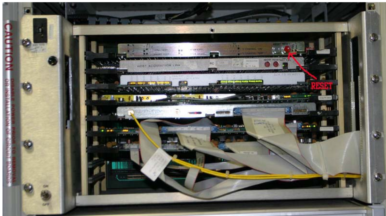
UNITY600 Plus Console RESET button position.
